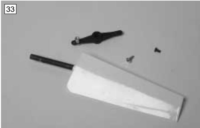
Locate the rudder and hardware to attach rudder.
