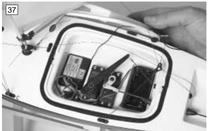
View of radio box with radio system installed
